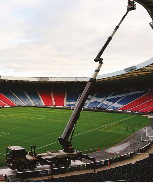
Built with the outstanding quality that we expect from Ruthmann the T460 has a working height of up to 46 m and an impressive outreach of up to 31 m. The 600 kg cage capacity can be utilised for lifting bulky materials using our electric duke winch.
