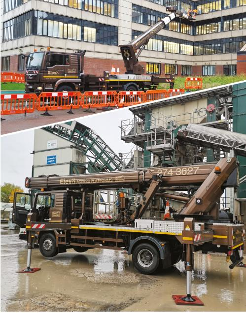
Built with the outstanding quality that we expect from Ruthmann the T380 has a working height of up to 38 m and an impressive outreach of up to 31 m. The 600 kg cage capacity can be utilised for lifting bulky materials using our electric duke winch.
