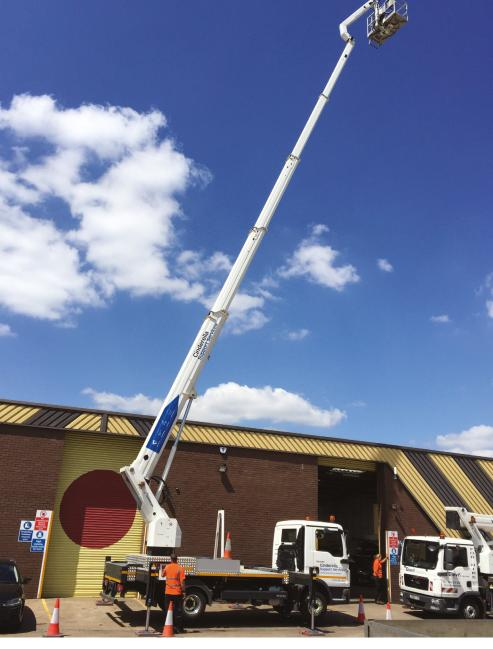
With 28.5 m of working height the TU285 is available for self-drive or operated hire. Built with the outstanding quality that we expect from Ruthmann the T285 has an impressive outreach of up to 20.5 m and a cage capacity of 320 kg.
