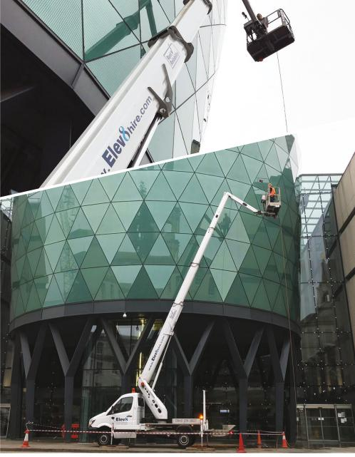
Mounted on a compact 3.5 ton truck the TBR220 is very easy to use, perfect for both self-drive and operated hire. Built with the outstanding quality that we expect from Ruthmann the TBR220 has an impressive outreach of up to 16.4 m and a cage capacity of 230 kg.
