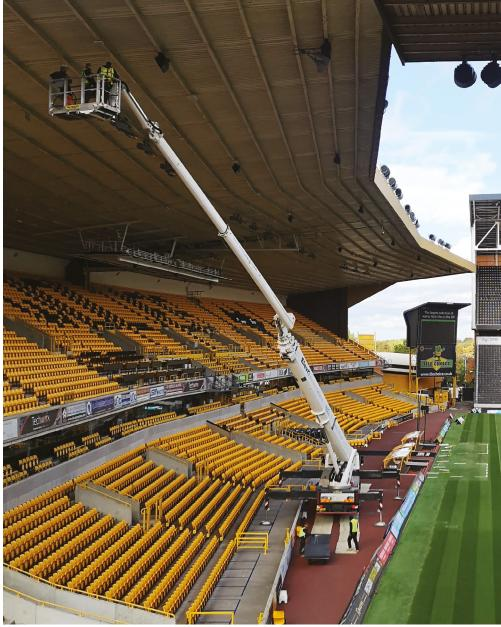
This MEWP has a hanging work cage which can rotate 2 x 200° to allow the full width of the cage to be used at the rear of buildings. With up to 15 m of negative reach this MEWP is ideal for bridge inspections. It has 600 kg safe lifting capacity.
