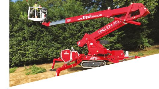
Compact and agile the LEO23GT is perfect for jobs with limited set-up space and complicated locations. It can be powered by either diesel or 230 V electric and has a transport width of just 0.98 m wide enabling it to fit through many entrance doors. The tracks have mechanically variable height adjustment so that it can be driven on slopes and the variable outrigger system allows it to be set-up in complicated locations.
