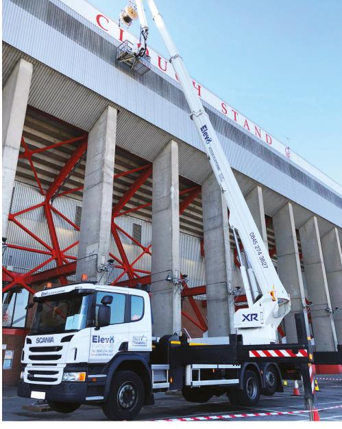
With up to 56 m of working height and 38.5 m of lateral outreach this MEWP has outstanding manoeuvrability. The S56XR can be utilised for lifting bulky materials using the wirelessly controlled 1300 kg boom winch or 400 kg cage winch.
